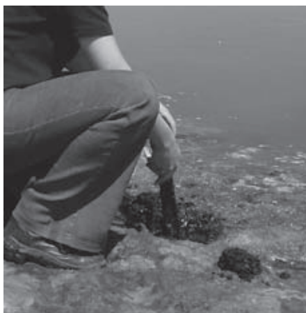
Sediment containing "monosulfidic black ooze" or MBO; the black material is likely to be rich in mackinawite and/or amorphous \text{FeS} .
